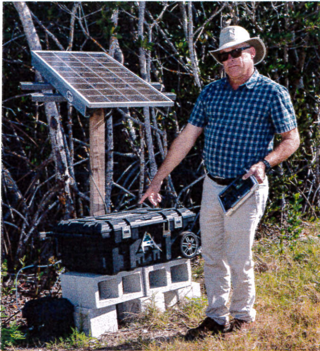
David Heuberger stands by a solar-powered data logger connected to antennas. This equipment tracks the fish coming and going through the adjacent exchange culvert.
